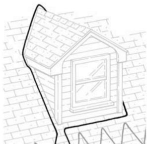
Figure 7. Cable pattern around a dormer
